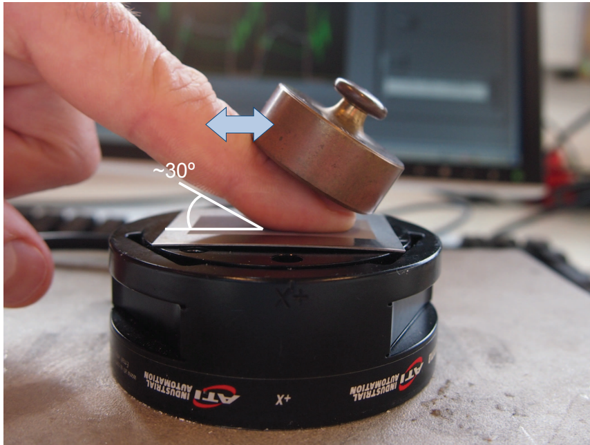
Figure 4. Experimental set-up for measuring the sliding friction between the fingerpad and textured samples.
